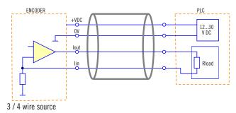
with 3 wires interface  $l_{\text{in}}$  is internally connected to  $0\mbox{\ensuremath{\text{V}}}$
