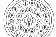
ME connector (32 pin) Glenair IPT 02 A 18-32 P F6 solder side view FV
